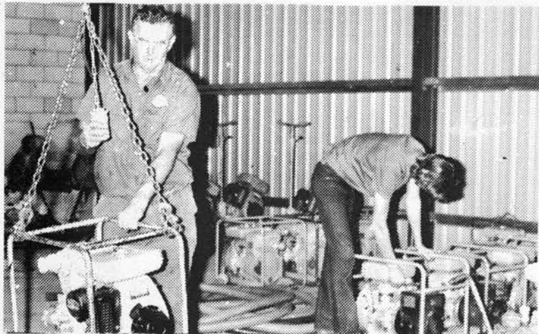
Jim Dormer showing how the electric chain hoist makes the lifting of heavy equipment within the workshop or when loading customer's vehicles "childs play".
